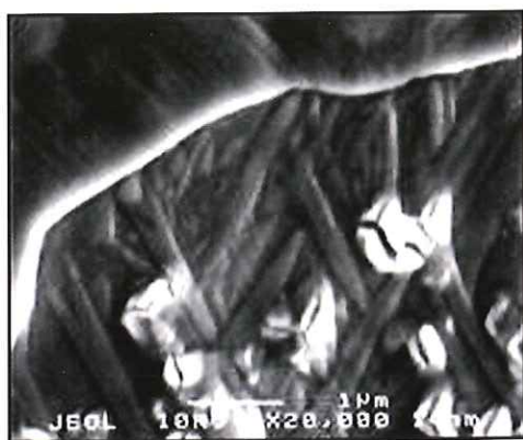
Figure 5: Thermal oxide on tantalum surface
