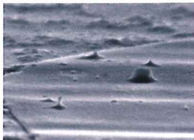
Figure 13: Crystalline nuclei on Ta surface inside anodic oxide film (x 20 000)
