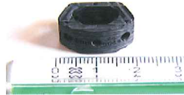
Figure 5: Human CFC Cage from Acromed-Depuy, model Brantigan PLIF (PLIF = Posterior Lumbar Interbody Fusion) was used for the study. (Ruler in foreground shows centimetres)
